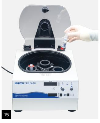
Ensure the appropriate counterweight and bucket spacers are in place.
