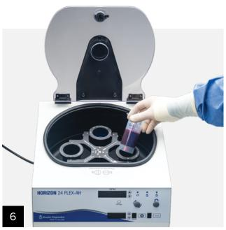
Open centrifuge lid. Place the ACP Max syringe into the centrifuge bucket.
