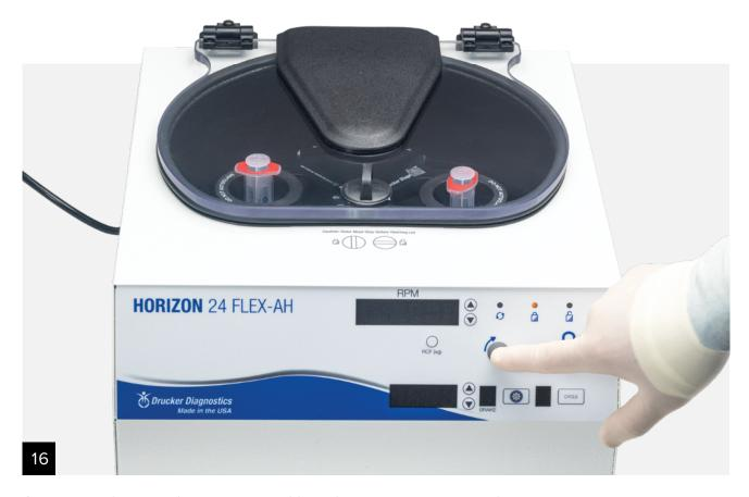
Close the lid of the centrifuge and set to 1500 rpm for 5 minutes. Begin centrifugation.
