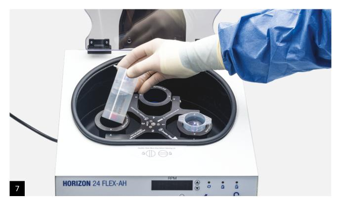
Using tap water, fill the ACP Max counterweight from the distal end to a volume equal to the ACP Max syringe. Ensure that the ACP Max counterweight is placed opposite to the ACP Max syringe within the centrifuge rotor. Set the centrifuge to the appropriate speed and time for processing volume. Begin centrifugation.
